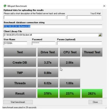
Benchmark results using Firebird 3.0 on an IFSML Server
