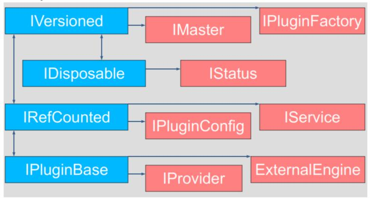
The base of the structure is **IVersioned**. It is the interface that enables a version upgrade. A lot of interfaces not requiring additional lifetime control are based directly on **IVersioned**. **IMaster** is one example already mentioned. Others include a number of callback interfaces whose lifetimes must match the lifetimes of the objects from which they were to be used for callback.
